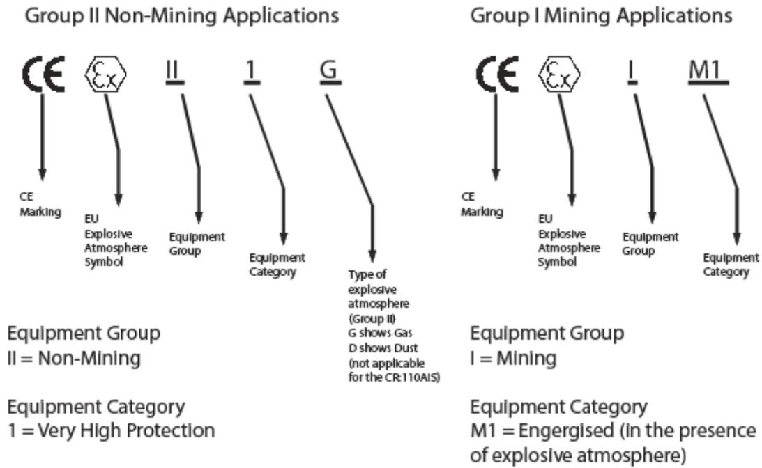
Because the ATEX Directive is different to the IEC/CENELEC Certification, different numbers are used for the Intrinsic Safety Approval. These are described below.
