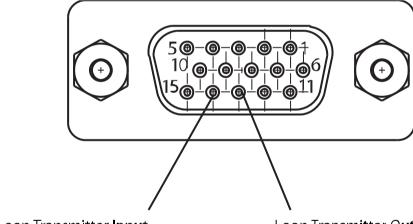
Loop Transmitter Input Pin14 Loop Transmitter Output Pin13
