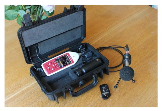
The Trojan<sup>2</sup> is an advanced noise nuisance recorder that has been designed to be simple to both setup and operate.
