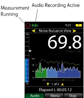
If the instrument has been left unattended for more than 15 minutes with the case closed, the display will be switched off to reduce power consumption. This can be changed in the NoiseTools software.
