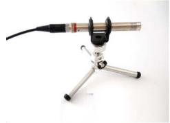
The case has a cut out that allows the preamplifier and the tripod mount to remain coupled when they are not being used.
