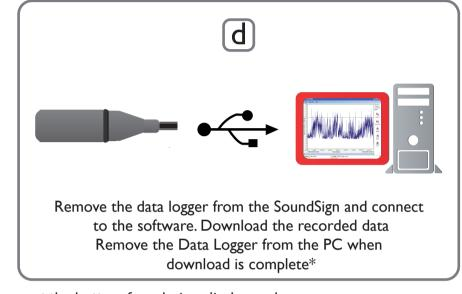
\*The Data Logger should be removed from the PC when not in use to prevent the battery from being discharged.
