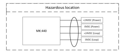
Wherever possible the MK:440 should be wired outside of any potentially explosive atmosphere. A single conductor must be used in each port.
