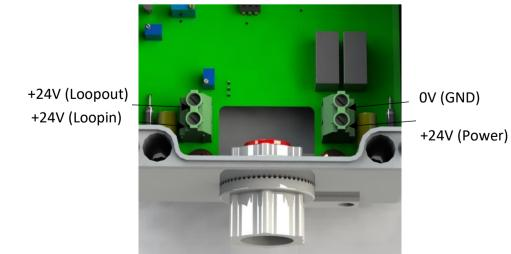
There must be no conductor extending beyond the terminal block, strip wires no more than 10mm.
