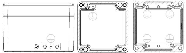
Note that the external and internal earths of the enclosure share an electrical connection, but the lid does not. Both parts of the enclosure must be connected to a suitable ground connection.
