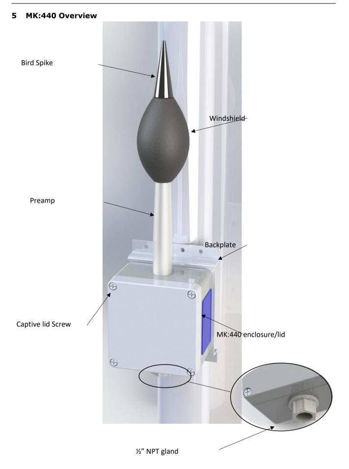
The standard version of the MK:440 has a 4-20mA current loop which outputs a current level, expressed in milliamperes that is proportional to the sound level with either a 'Fast' or 'Slow' Time Weighting. The choice of time weighting is a factory set option made at the time of purchase.
