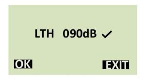
Set the desired level and enabled the alarm by using the arrow buttons. A tick denotes that the alarm is active; a cross denotes that the alarm is disabled. When set, press (a) to confirm.
