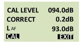
Use the arrow keys to set the CAL LEVEL to the acoustic calibration level (94.0dB for the CR:514 calibrator).
