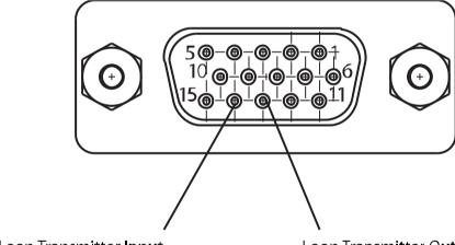
Loop Transmitter Input Pin14
